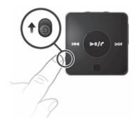
• Move the switch upwards.
